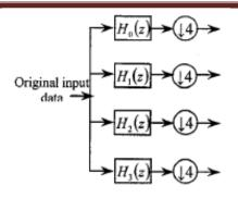
**Fig.1**: (b) Two-scale filterbank structure using the SLT.
